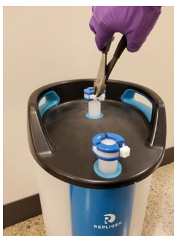
Figure 4. SaniSure® Clamp Removal
