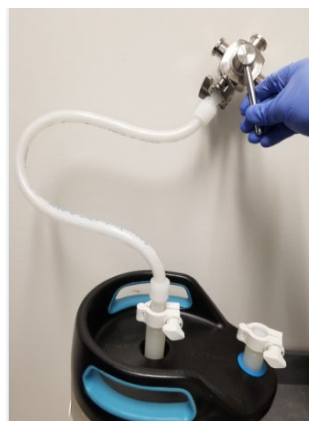
Figure 5. Stainless Steel Valve Connection to OPUS® Column
